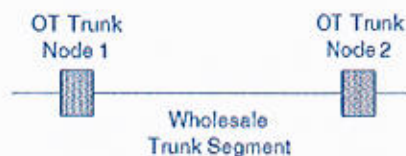
Figure 3-1 Trunk Segment of Leased Line
